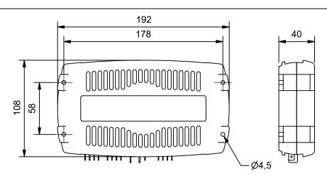
Item no. Voltage Wipers 532212 12/24 V Up to 2 532213 12/24 V Up to 3 532214 12/24 V Up to 4 532215 12/24 V Up to 5
